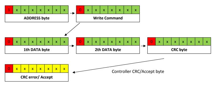
Every ADDRESS byte MSB bit must be "1" any other which is not an ADDRESS byte must be "0".
