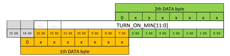
Turning On Minimum voltage register sets the voltage level where the controller will turn back from low supply status if the supply voltage is higher than the register value. With default settings it is disabled in the controller.Writing and locking this register activates the function.
