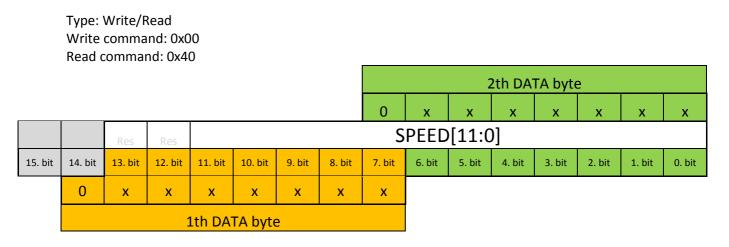
Speed register gives the base value of the output voltage (duty cycle). The final value depending some other factors. The final duty cycle depending on several other factors (current limits, regen modes..)
